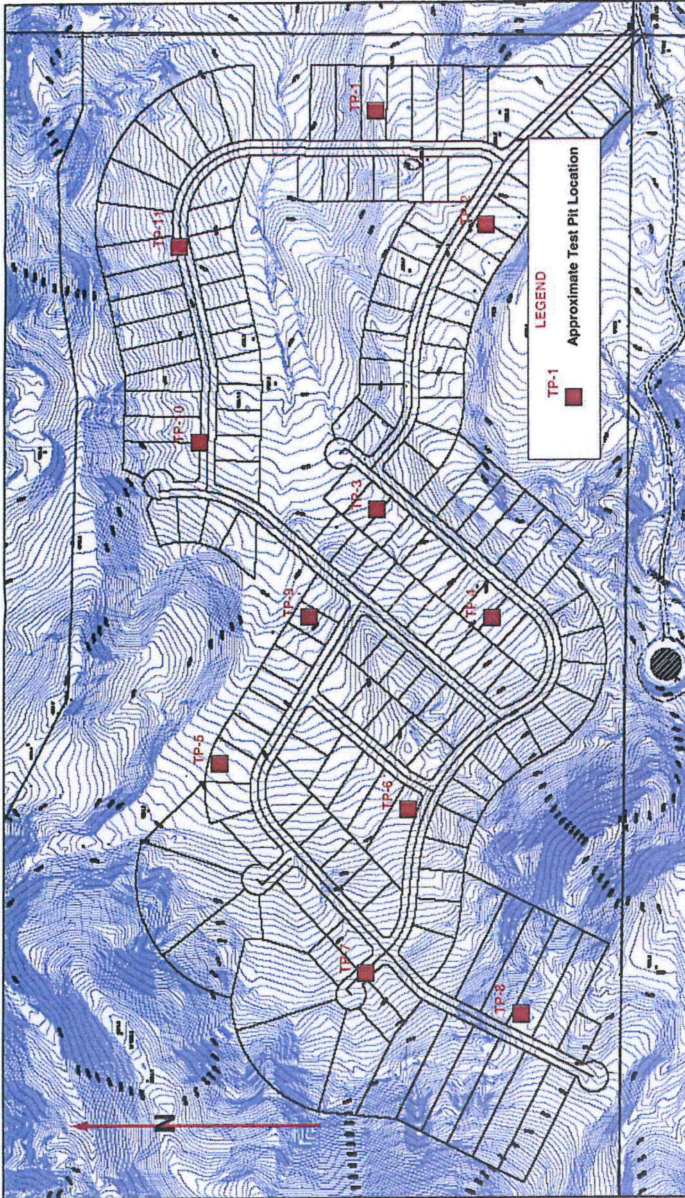
SITE PLAN AND APPROXIMATE TEST PIT LOCATIONS
